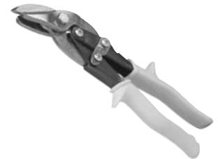
\*When cutting laminates, the finished surface should be on the side of the center blade to avoid excessive cracking.
