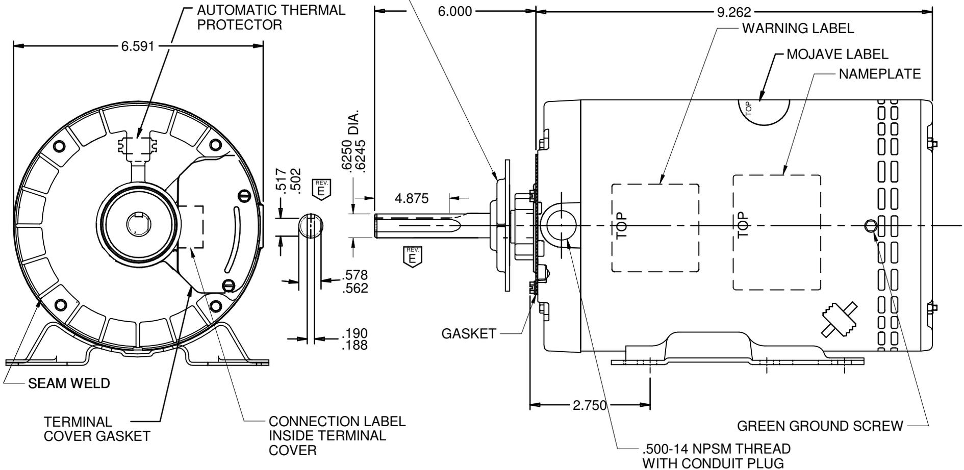
SHAFT KEY TAPED TO MOTOR
