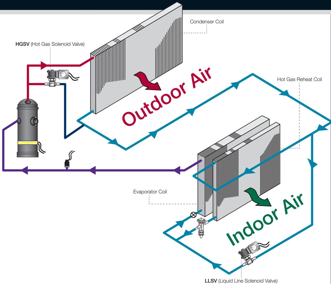
This two-phase mixture is routed through the unit's coil and then the evaporator. Additional sub-cooling of the refrigerant occurs in the coil, and when this refrigerant is fed into the evaporator, the result is a colder coil surface.
