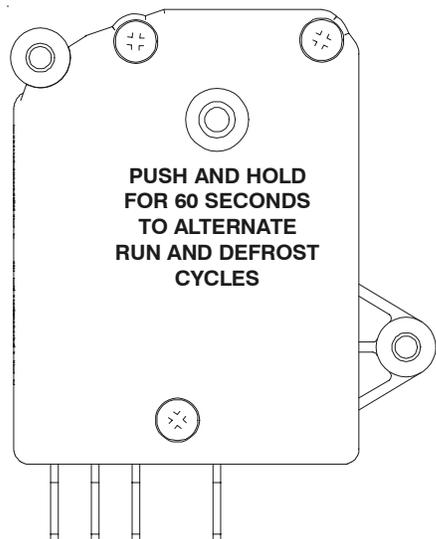
Some refrigerators do not use plug-in connectors for a defrost timer hook-up. Each terminal is connected using a separate wire. In this case, very carefully bend terminals 2, 4, 3 as illustrated. Use needle-nose plier to hold the terminal while bending it with another plier.
