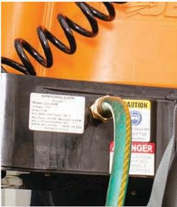
Standard hose connector for continuous water supply
