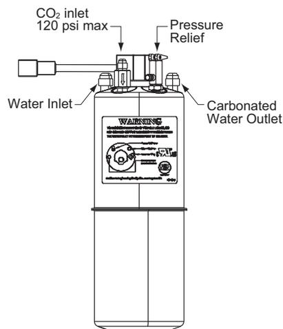
The carbonator is replenished when the carbonated water level inside the tank drops, which in turn automatically starts the carbonator water pump. When the water level inside the tank has been replenished, carbonator water pump will stop.
