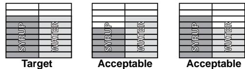
9. Adjust dispensing valves for water-to-syrup ratio (brix) as recommended by the syrup distributor.
