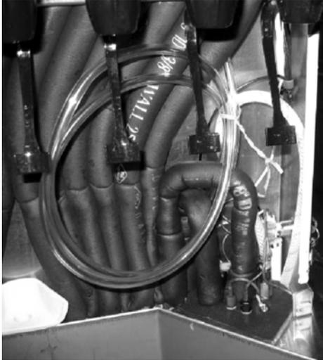
2. Purge tube is connected to the pressure relief valve on carbonator tank and must be routed to a drain. Route carbonator tank purge tube (A) down through the valve leads conduit, which is located behind the carbonator tank. Be sure not to collapse or kink carbonator tank purge tube during routing from unit to drain.
