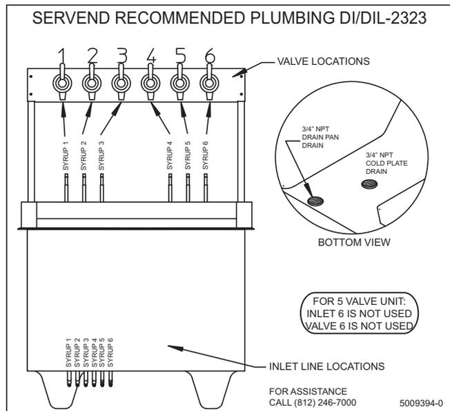
**Internal Carbonator Connections**
