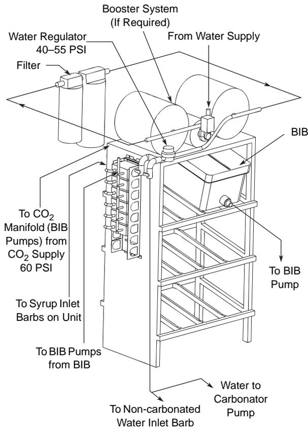
1. **Incoming tap water** - should be at a minimum dynamic pressure of 40 psi and maximum static pressure of 55 psi.
