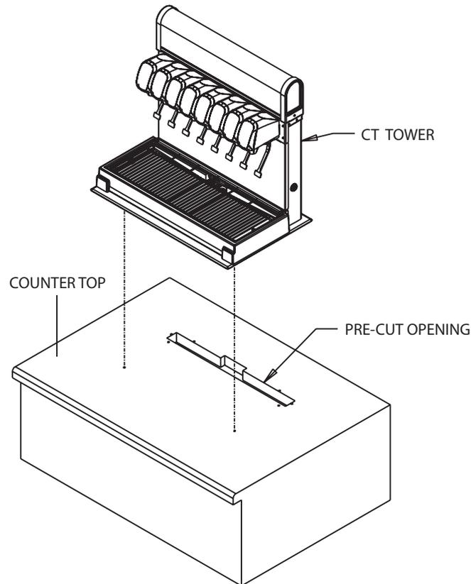
1. Remove drain pan grid, splash panel and drain pan before installation.
