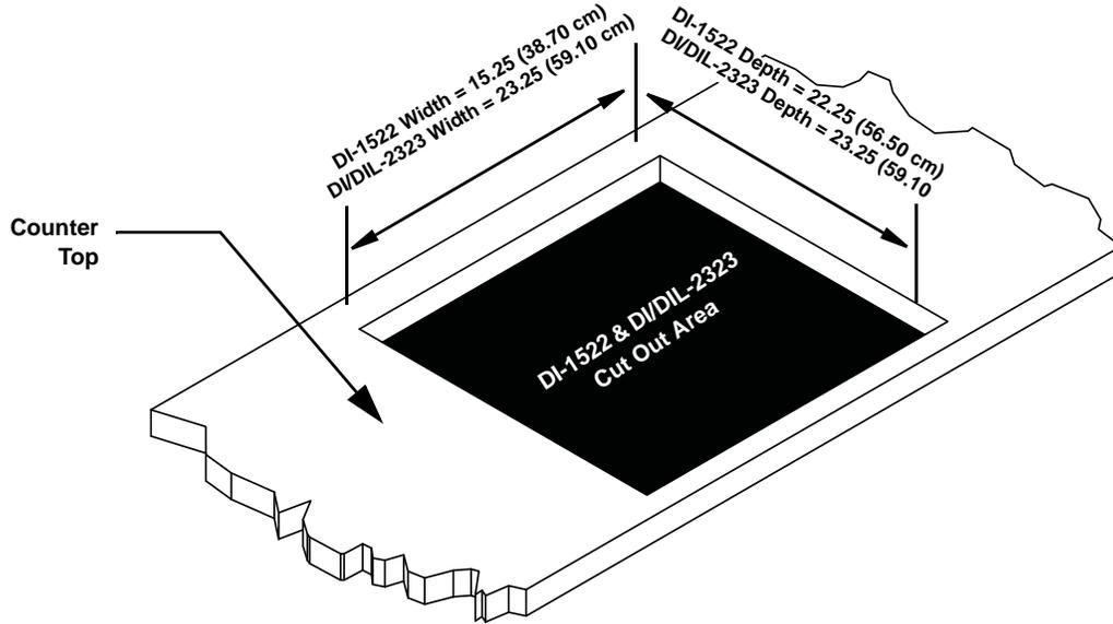
1. Mark the counter top with the appropriate cut out opening dimensions, see illustration above.
