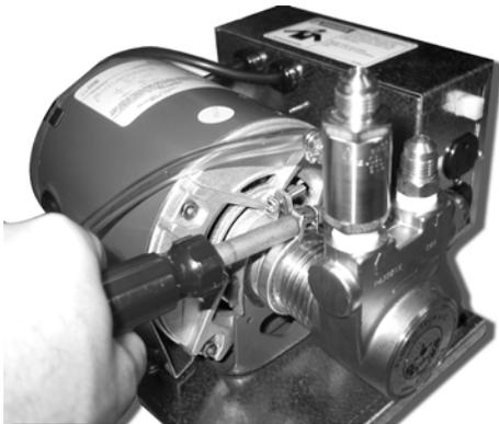
2. Turn the pump to the position shown and secure in place by re-tightening the clamp screw.
