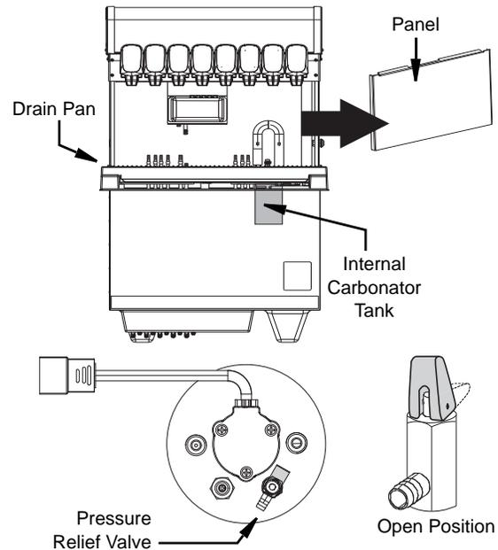
3. Turn on the water to the unit, fill the carbonator with water and close the vent on the carbonator pressure relief valve when water begins to escape the vent.
