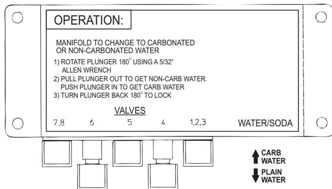
Illustration above shows the Carbonated position. Make adjustments using a 8 mm wrench or socket. Turn 180° clockwise to switch the beverage to Non-carbonated Water.
