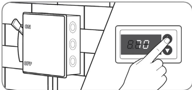
With thermostat in the "Off" position, turn the power on to the furnace or air handler and the heat pump. Start the heat pump and the furnace or air handler with the thermostat. Verify that the outdoor unit is operating in second stage and the indoor air mover is delivering the second-stage airflow for the system size.
