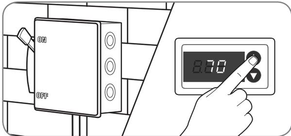
With thermostat in the “Off” position, turn on the power to the furnace or air handler and the heat pump. Start the heat pump and the furnace or air handler with the thermostat. Verify that the outdoor unit is operating in second stage and the indoor air mover is delivering the correct airflow for the system size.
