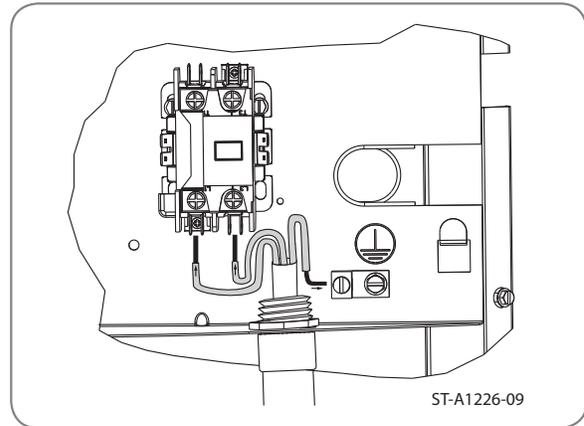
A grounding lug is provided near the line-voltage power entrance for a ground wire.
