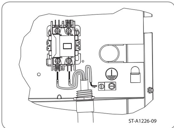
Connect power wiring to line-voltage lugs located in the outdoor heat pump unit electrical box. (See wiring diagram attached to unit access panel.)
