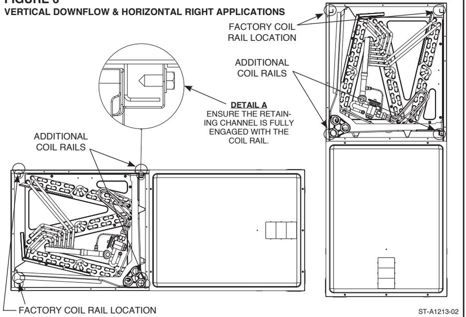
**FIGURE 7****INDOOR COIL AND DRAIN PAN DETAILS**
