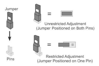
• Control adjustment is now restricted to changing only the OFF value, which shifts the On and OFF control band within the restricted adjustment range defined by HtS and LtS.
