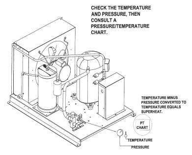
**DETERMINING COMPRESSOR SUPERHEAT**
