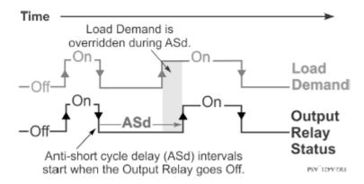
• Anti-short cycle delay is typically used for refrigeration applications so that the system pressure can equalize before restarting the compressor.
