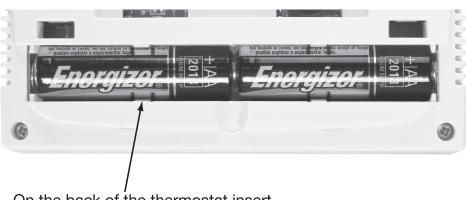
On the back of the thermostat insert 2 AA Alkaline batteries (included).
