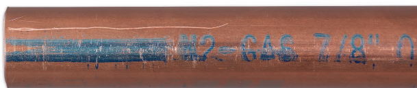
Figure 2 - Copper tube with “bad” surface scratch.
