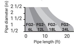
Add 1 foot to your pipe length for each valve or spigot on your pipe system. If cable selected is longer than the pipe, spiral it evenly along the entire pipe.
