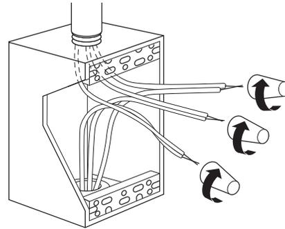
**Connecting the FrostGuard cable to power**
