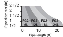
Add 1 foot to your pipe length for each valve or spigot on your pipe system. If cable selected is longer than the pipe, spiral it evenly along the entire pipe.
