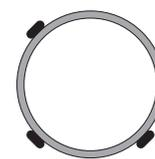
1d Three cables in 4, 8, and 10 o'clock positions
