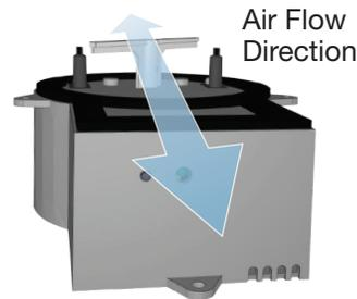
1. The iWave-R has universal voltage capability, connect 24VAC to 260VAC voltage input, whatever is most convenient for quick installation. Although the device only pulls 10 watts, sometimes a dedicated 24VAC power supply may be necessary depending on the current load on the transformer for other system accessories.
