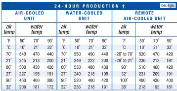
†Production for Dice and Half Dice cubes. Data is published for 60 Hz machines. 50 Hz machines produce approximately 7% less ice.
