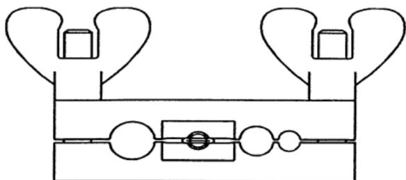
FIG. A - "PINCHING OFF" TUBING
