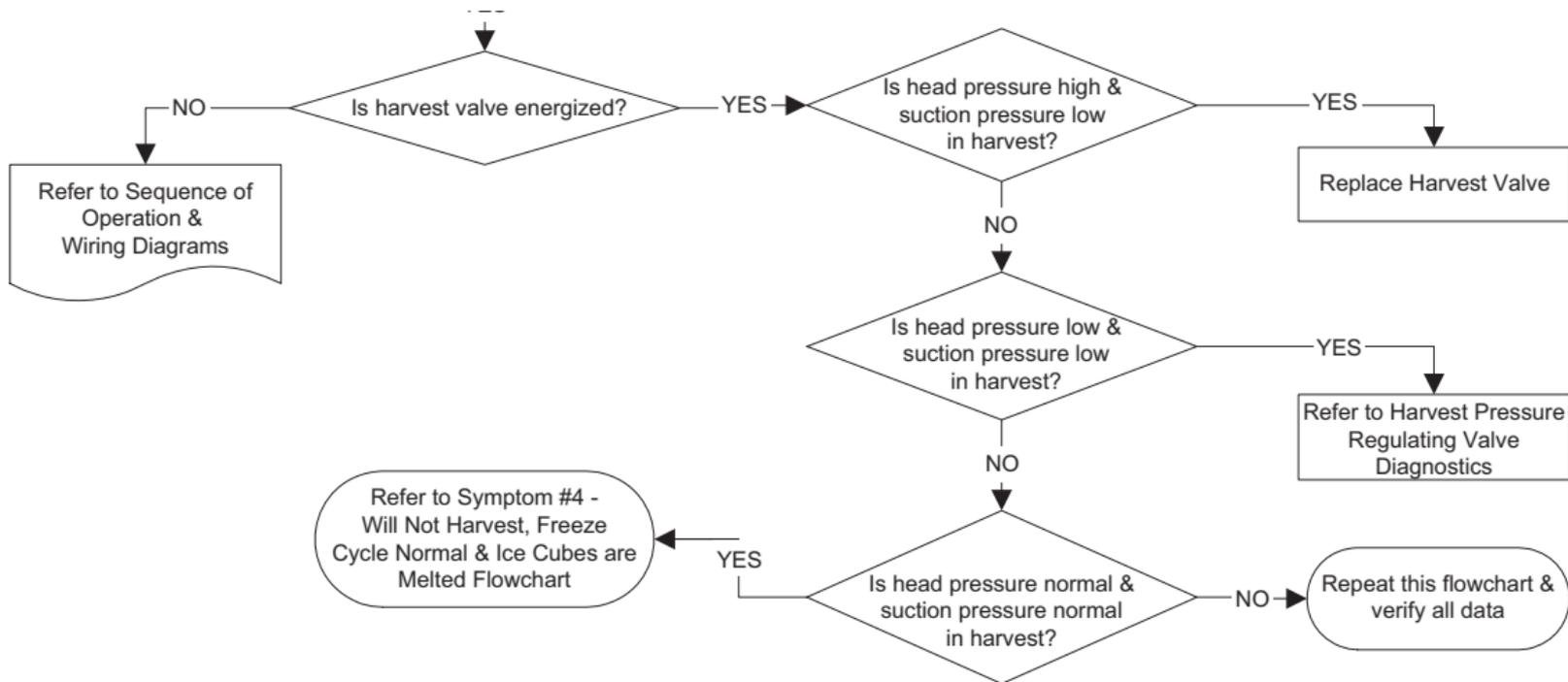
*Single Evaporator Systems with Dual Harvest Valves: If one Harvest Valve is open and the other is restricted / stuck closed you may have normal harvest pressures. Look for ice not melting on one side of the evaporator.*
