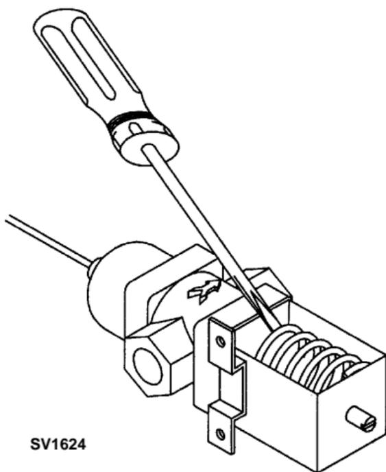
4. Hold the valve open and blow compressed air through the condenser until no water remains.
