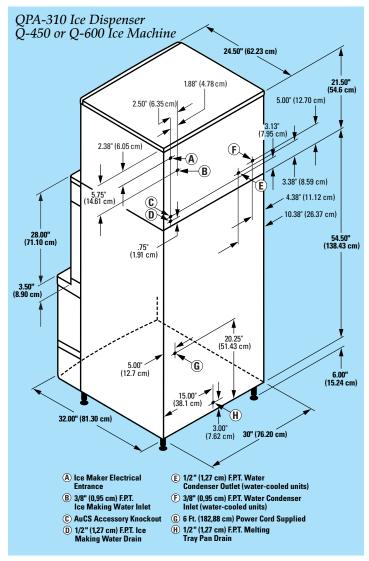
*Installation Note* - Dispensers have no minimum clearance, when installing an ice machine/dispenser combination follow the clearance requirements for the ice machine being installed.
