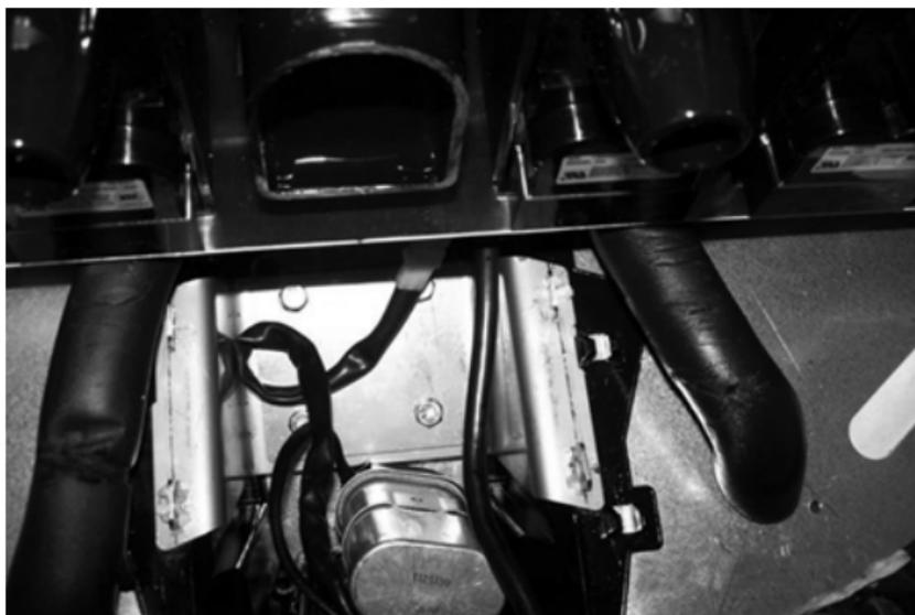
6. New motor must have the same alignment (within 15 degrees).
