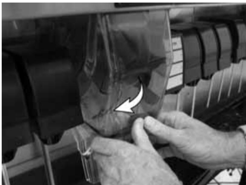
C. Rock top of the chute forward until top of chute clears unit.
