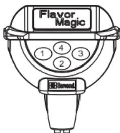
To line up flavors with valves, note that valve outlets number from left to right 1...2...3...4. Touch pad flavor tab is numbered as shown below. Connect vinyl tube from outlet 1 and dispense with flavor tab 1, etc.
