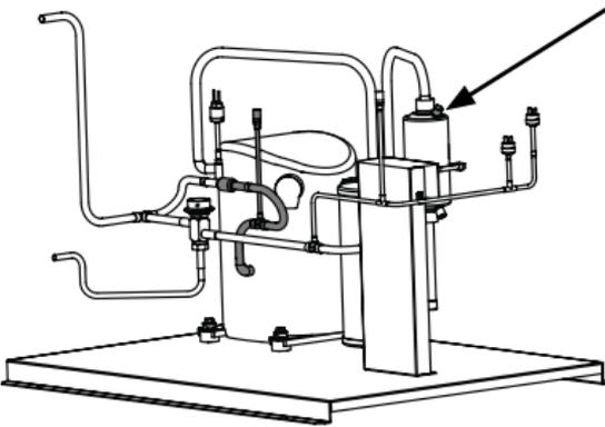
Connections must also be made at two points on condensing unit for complete refrigerant recovery.
