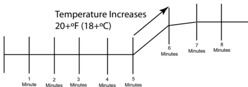
The time needed to remove the liquid refrigerant will vary with the ambient temperature and the length of the harvest cycle. Higher ambient temperatures = shorter harvest cycles, faster removal of liquid refrigerant from the accumulator and greater suction line temperature increases.
