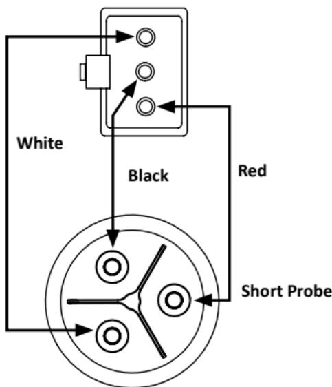
**Ohm water Level Probe and Wiring Harness**
