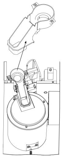
15. The ice chute can be cleaned in place. If complete removal is desired, use a Phillips screwdriver to remove the Hall Effect switch assembly from the ice chute.
