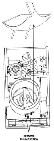
19. Remove ice dispensing wheel by lifting straight out.
