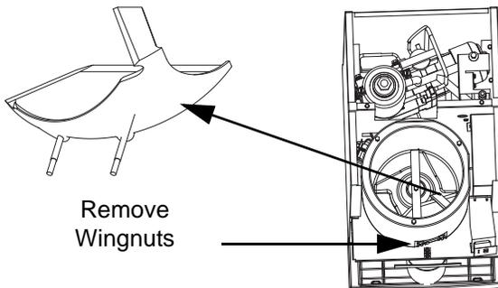
18. Remove ice dispensing wheel by lifting straight out.
