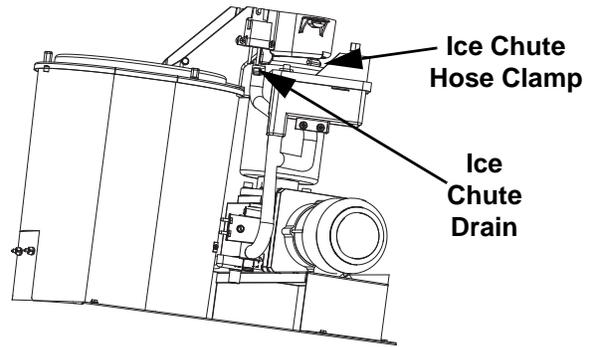
13. Lift up on ice chute to remove. The ice chute must be removed before the bin cover can be removed.
