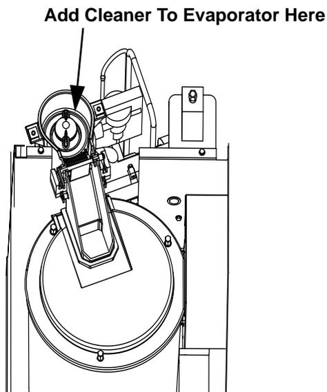
**Step 3** The ice machine will run a wash cycle, a series of rinse cycles and then stop. This entire cycle lasts approximately 30 minutes.
