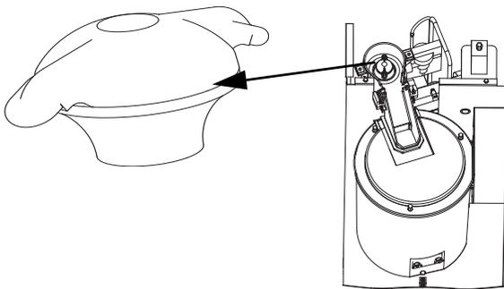
11. Loosen ice chute hose clamp.
