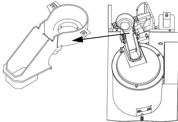
14. The ice chute can be cleaned in place. If complete removal is desired use a phillips screwdriver to remove the Hall Effect Switch assembly from the ice chute.
