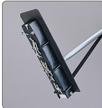
Powerful Magnetic Surface efficiently picks up debris.
