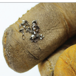
Easily Remove Metal Shavings from Magnetic Tip
