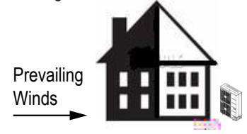
Figure 45: Leeward Side of the Building.
