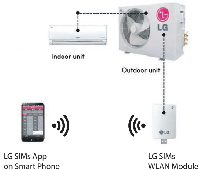
Figure 83: SIMS WLAN Module to DFS System Example.
