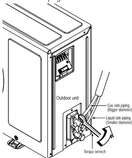
Figure 43: LSU180HEV1 Outdoor Unit Piping Connection.
