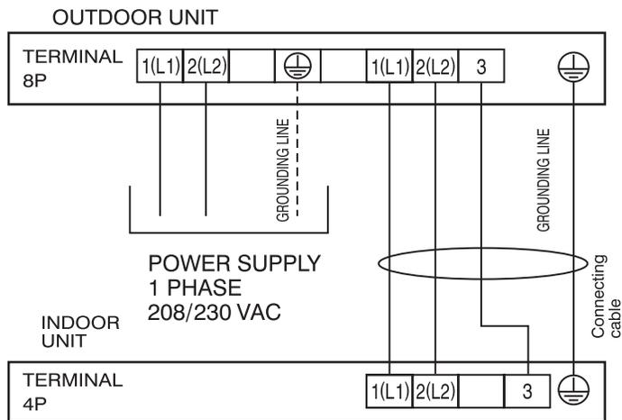
Figure 53: Terminal Block Wiring Diagram LS090HXV, LS120HXV
