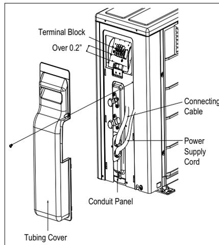
Figure 48: LSU240HEV1 Outdoor Unit Electrical Connection.
