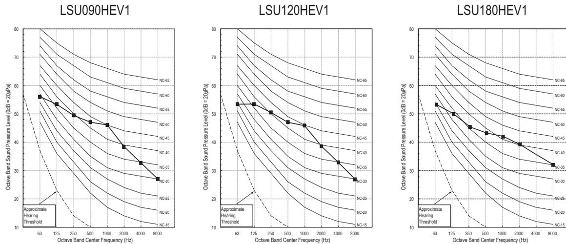
Figure 3: Sound Pressure Levels for Mega 115V Outdoor Units.
