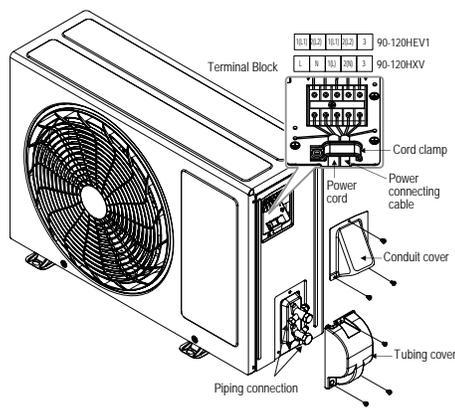
Figure 47: LSU180HEV1 Outdoor Unit Electrical Connection.
