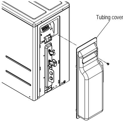
Figure 40: LSU240HEV1 Outdoor Unit Connection Cover Removal.
