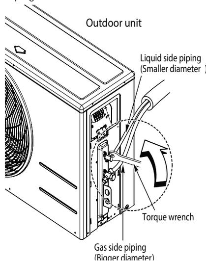
Figure 44: LSU240HEV1 Outdoor Unit Piping Connection.
