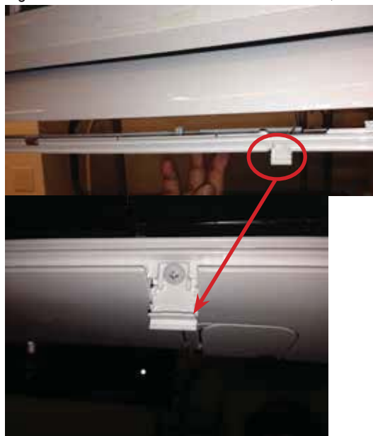
Figure 88: Remove Screws from Bottom Panel
