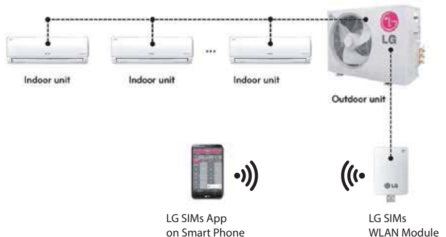
Figure 114: SIMs WLAN Module to Typical DFS System
