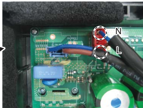
< Main PCB wiring Check Point >
