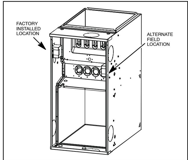
**Figure 24 – Field-Supplied Electrical Box on Furnace Casing**
