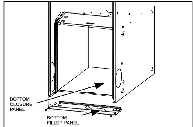
2. Rotate bottom filler panel downward to release holding tabs.
