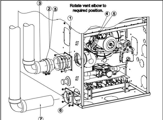
Rotate vent elbow to required position.
