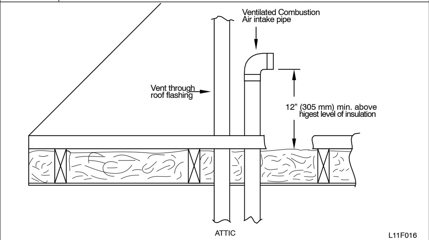
**Figure 57** Direct Vent Termination Clearance
