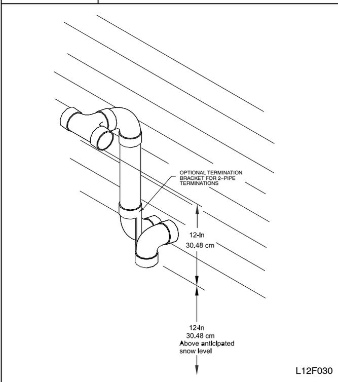
**Figure 45 Sample Inlet Air Pipe Connection for Polypropylene Venting Systems**
