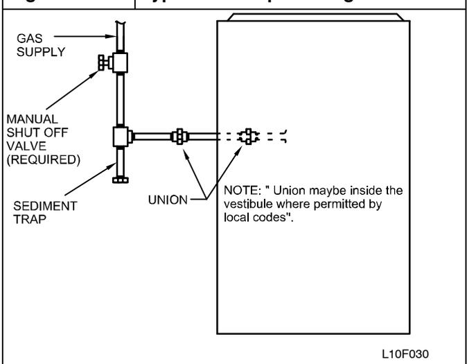
A 1/8-in. (3 mm) NPT plugged tapping, accessible for test gauge connection, **MUST** be installed immediately upstream of gas supply connection to furnace and downstream of manual equipment shutoff valve.
