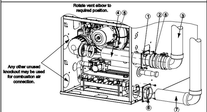
Rotate vent elbow to required position.
