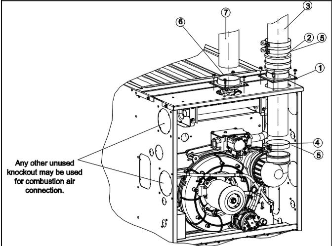
Any other unused knockout may be used for combustion air connection.
