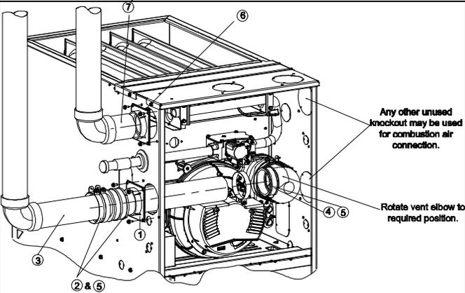
Any other unused knockout may be used for combustion air connection.
