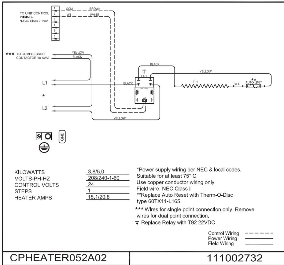
Fig. 15 - CPHEATER052A02 Wiring Diagram
