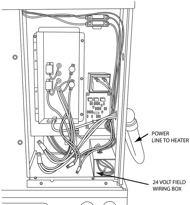
**Fig. 7 - Single Point Connections for Non-Fused Heater**
