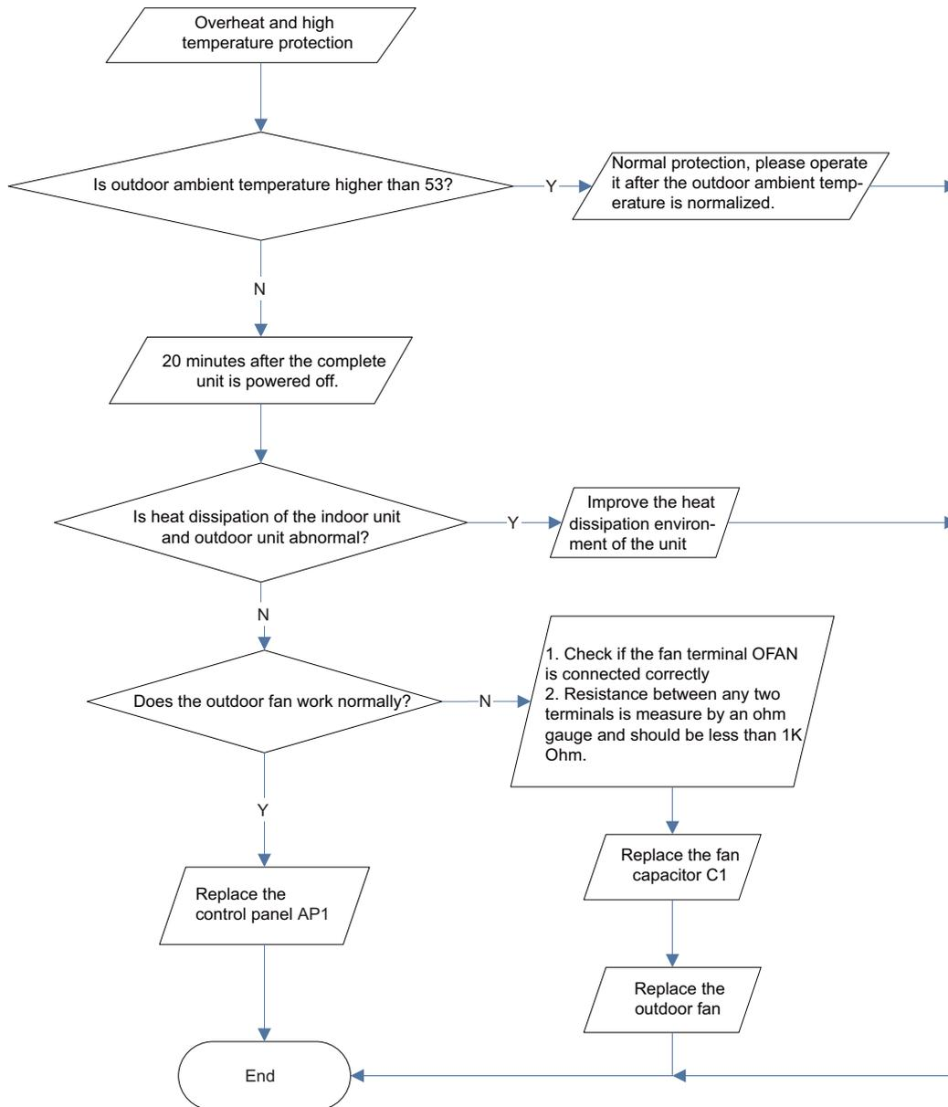
(4) Start-up failure (following AP1 for outdoor unit control board)
