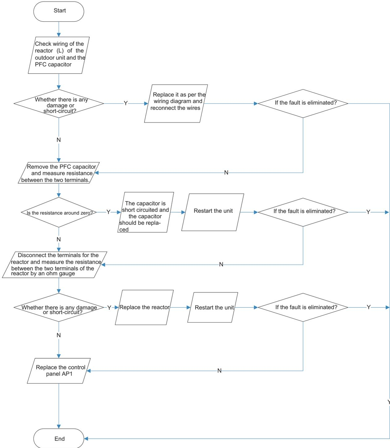
(8) Communication malfunction: (following AP1 for outdoor unit control board)
