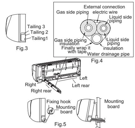
**7.3.6 Installation of Connection Pipe**
