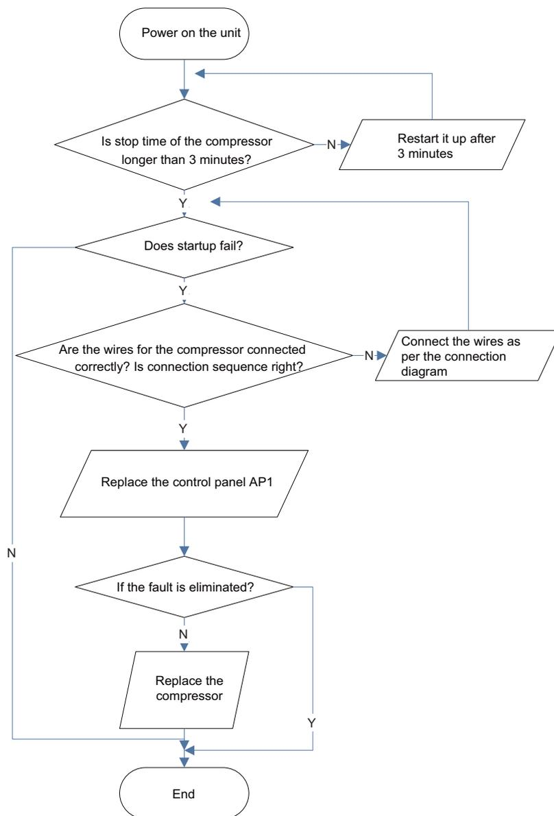
(5) Out of step diagnosis for the compressor (AP1 hereinafter refers to the control board of the outdoor unit)
