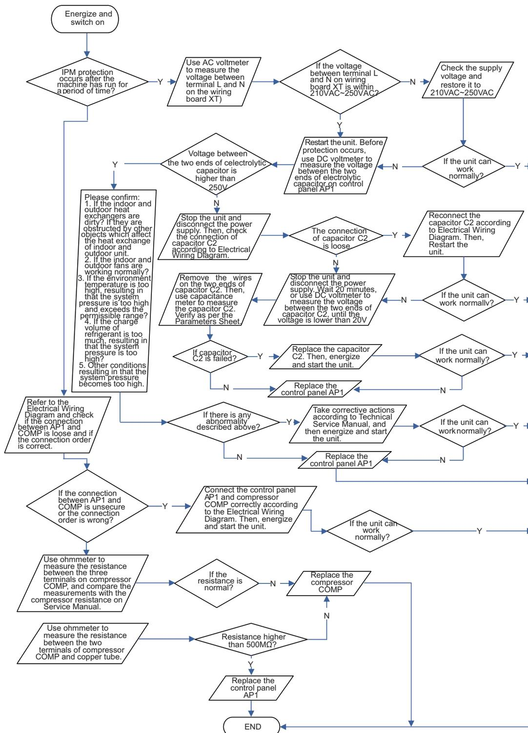
(3)High temperature and overload protection diagnosis (AP1 hereinafter refers to the control board of the outdoor unit)
