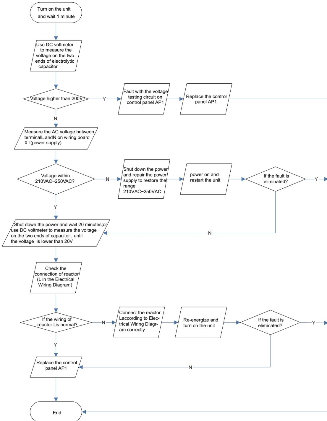
(2) IPM Protection, Out-of-step Fault, Compressor Phase Overcurrent (AP1 below refers to the outdoor control panel)
