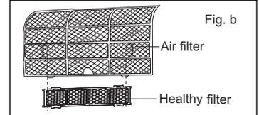
3. Install the air filter properly along the arrow direction in Fig.c, and then close the panel .
