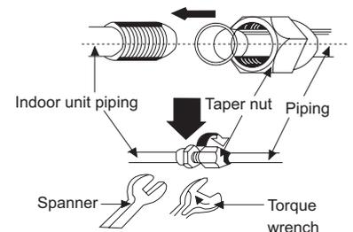
NOTE: Connect the connection pipe to indoor unit at first and then to outdoor unit. Handle piping bending with care. Do not damage the connection pipe. Ensure that the joint nut is tightened firmly, otherwise, it may cause leakage.
