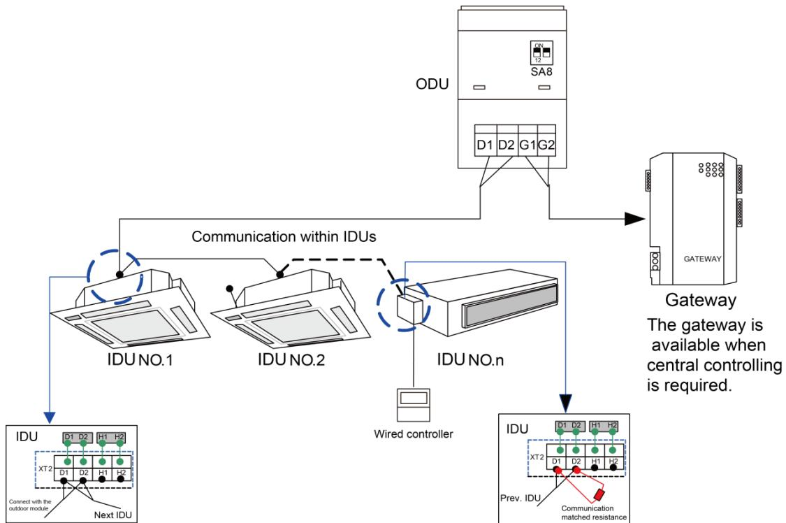
Fig.51 Connection of single unit
