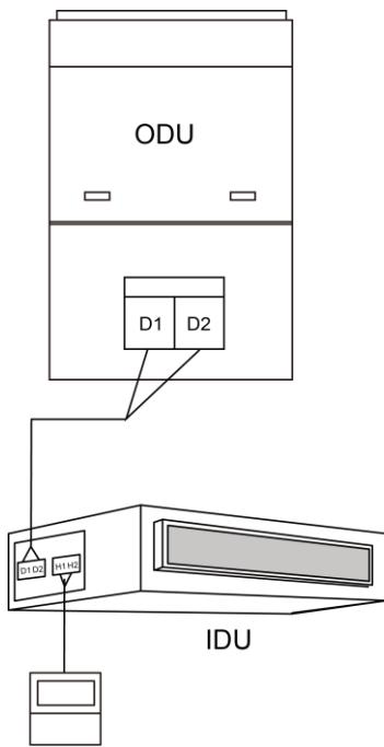
Fig.53 one wired controller controls one IDU
