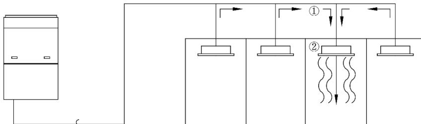
① Flow direction of refrigerant leakage.
