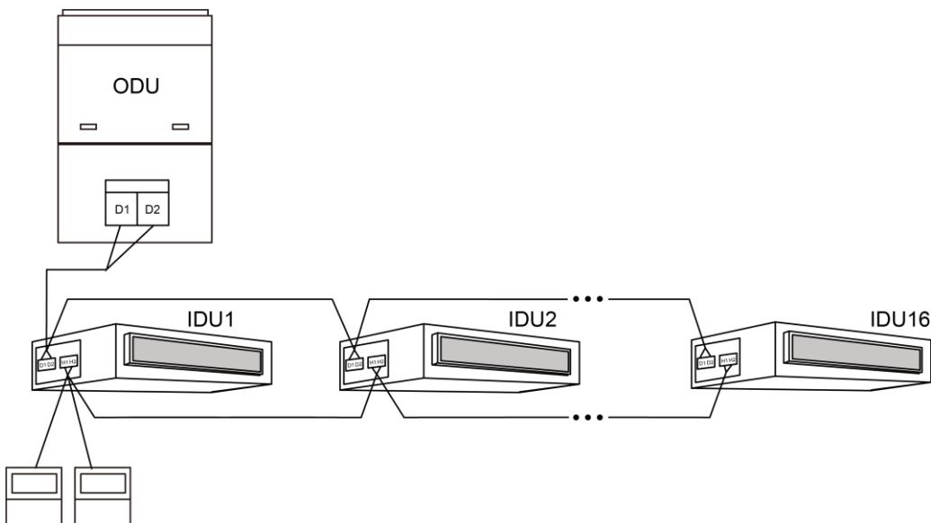
Fig.56 Two wired controllers control multiple IDUs
