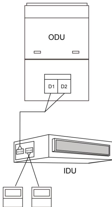
Fig.54 Two wired controllers controls one IDU
