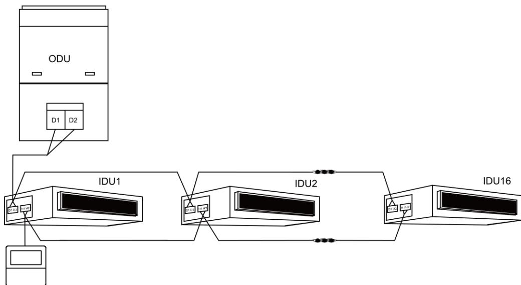
Fig.55 one wired controller controls multiple IDUs
