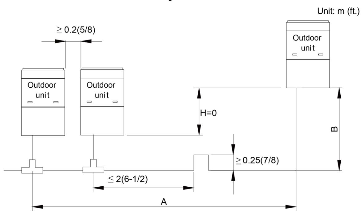
**NOTICE!** When the distance between outdoor units exceeds 2m (6-1/2ft.), U-type oil trap should be added at low-pressure gas pipe.  $A+B \leq 10m$  (32-7/8ft.).
