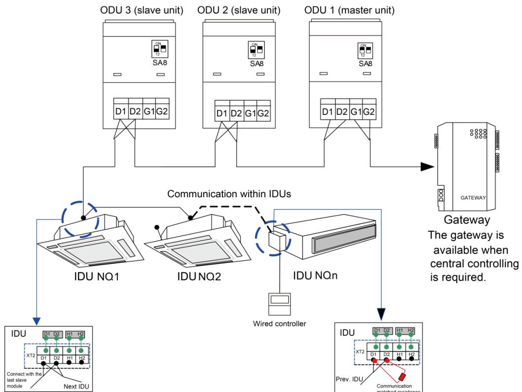
Fig.52 Connection of modular unit
