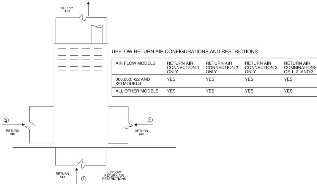
**Fig. 19 - Upflow Return Air Configurations and Restrictions**
