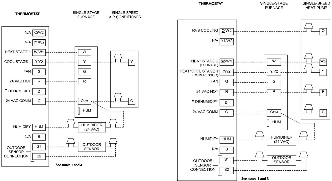
**Single-Stage Furnace with Single-Speed Air Conditioner**
