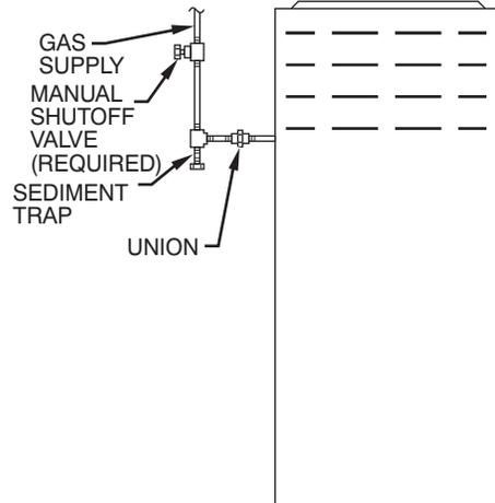
**Fig. 18 - Typical Gas Pipe Arrangement**
