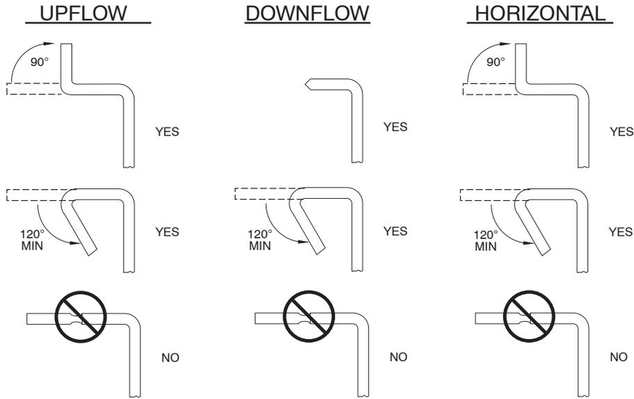
**Fig. 14 - Duct Flanges**
