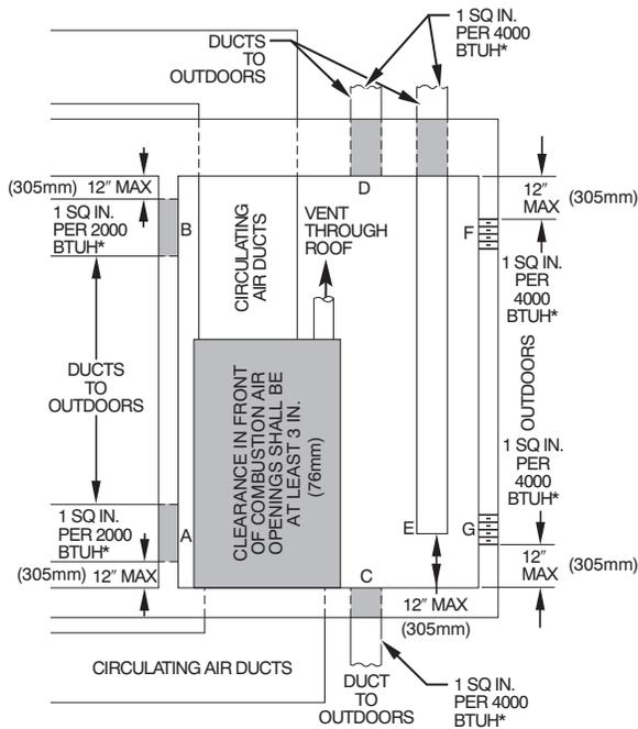
\*Minimum dimensions of 3 in. (76 mm).
