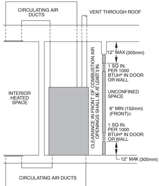
\*Minimum opening size is 100 in.<sup>2</sup> with minimum dimensions of 3 in. (76 mm).
