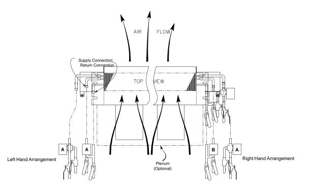
Figure 1 - Determination of Right-hand/Left-hand References
