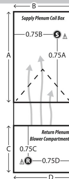
Recommended hole placement for SUPPLY measurement.
