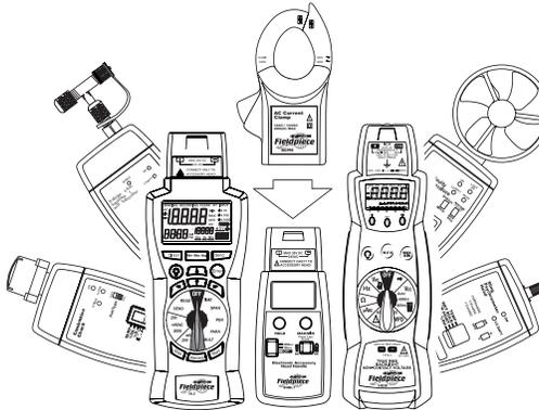
Accessory heads (the sensors) send a mV signal, which represents the value of the parameter being tested. Heads can attach directly to the top of a Stick meter, DL3 data logger, or EHD1. They can also plug into any meter with mV ranges using ADLS2 leads.
