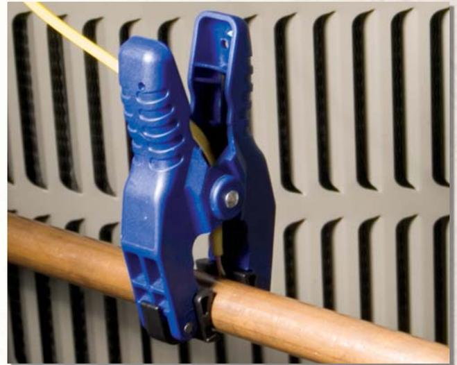
Figure 15. ATC1 pipe clamp thermocouple attached to a pipe correctly.
