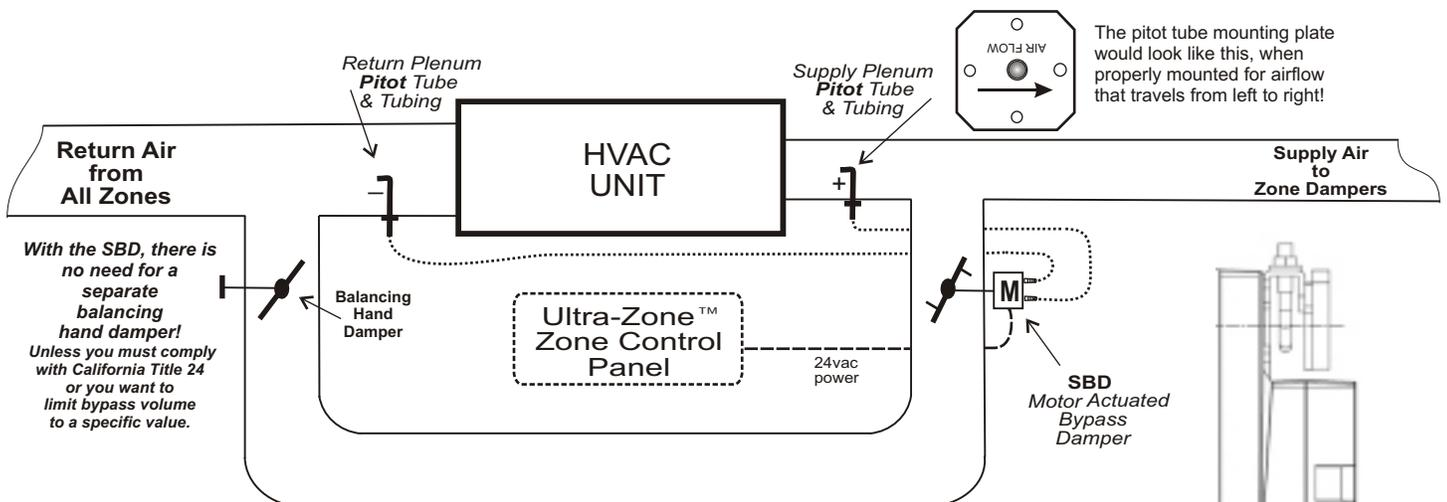
**Note:** This drawing of the Smart Bypass Damper and bypass duct work is intended to serve as a guide. Your actual duct configuration may differ. Just make sure all components are installed and setup correctly. If required, call EWC Controls Technical Support for assistance.
