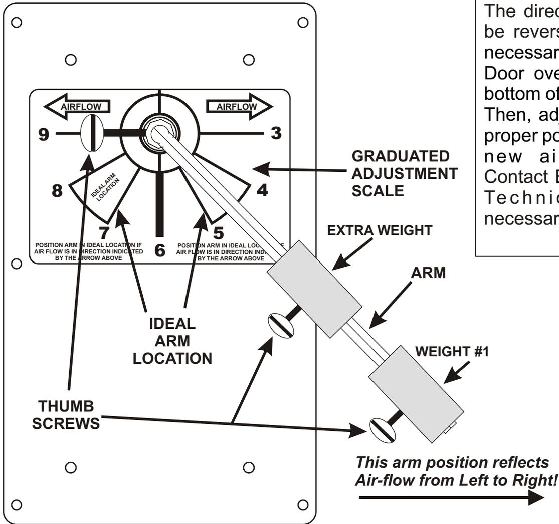
The direction of airflow can be reversed on the PRD if necessary, by pushing the Door over the stop on the bottom of the damper frame. Then, adjust the arm to the proper position based on the new airflow direction. Contact EWC Controls Inc., Technical support if necessary for further details.
