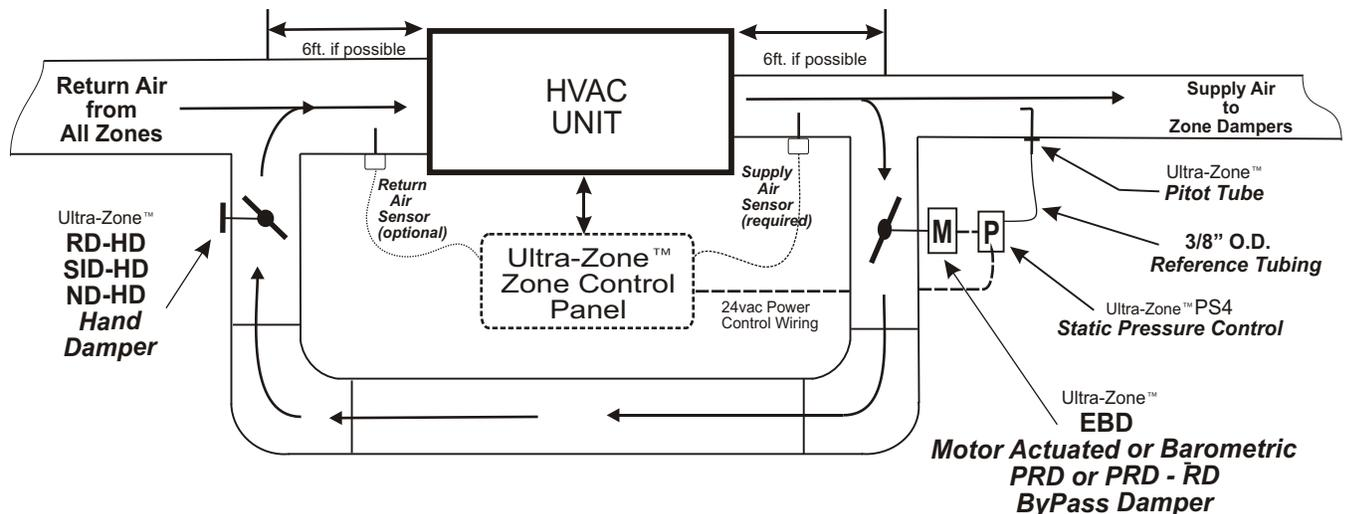
Note: This drawing of the Bypass damper, Hand Damper, Static Pressure control and Related duct work is intended to serve only as a guide. Your actual duct work layout and components may differ. Use the graphic as a guide when planning or designing a Zone system regardless of the Equipment type, Duct layout and Airflow configuration.
