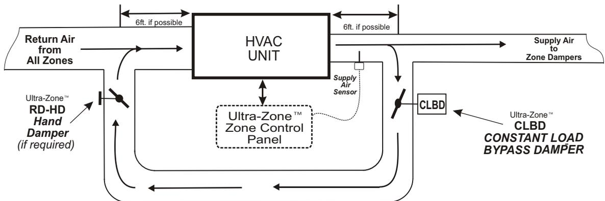
**Note:** This drawing of the Bypass damper, Balancing Hand Damper, and Related duct work is intended to serve only as a guide. Your actual duct work layout and components may differ. Use the graphic as a guide when planning or designing a Zone system regardless of the Equipment type, Duct layout and Airflow configuration.
