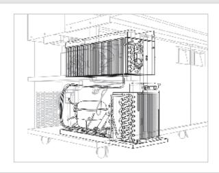
Space and accessibility is vital to the proper care and maintenance of equipment. The side-mounted condensing unit is designed with this in mind. The front grill unlatches with ease to reveal the condensing unit chamber. The entire carriage slides out in just a few easy steps for unrestricted access to the refrigeration components.
