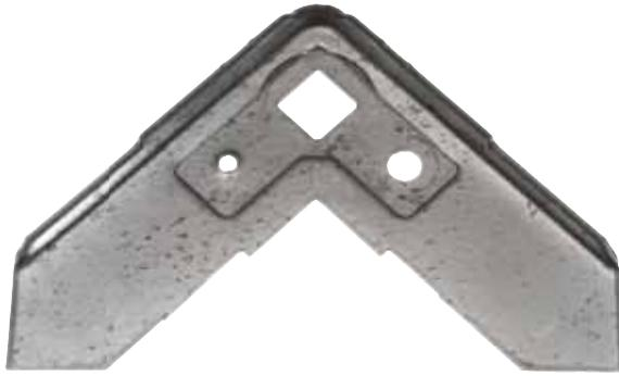
The Nexus J Corner is a galvanized steel product that is flanged and embossed to provide strength and rigidity. The corner piece has a square bolt hole to accommodate compatible carriage bolts allowing field assemble with a single wrench. Corners are pre-punched to accommodate #10 sheet metal screws.
