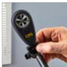
Thumbwheel for attaching/removing threaded universal end
