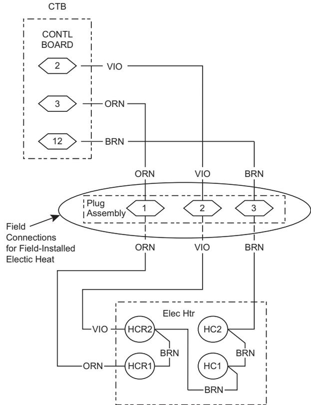
**Fig. 32 — Accessory Electric Heater Control Connections**
