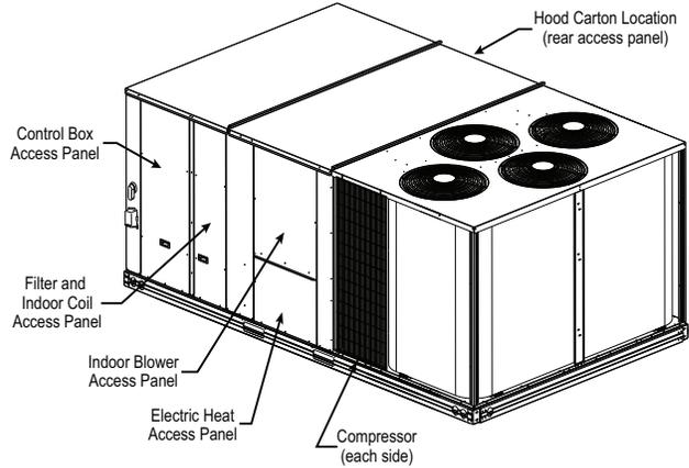
**Fig. 7 — Typical Access Panel and Compressor Locations**
