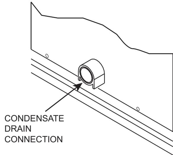
**Fig. 17 — Condensate Drain Pan Connection**
