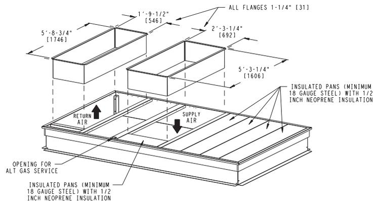
Fig. 9 — Roof Curb Details — RAH210-243
