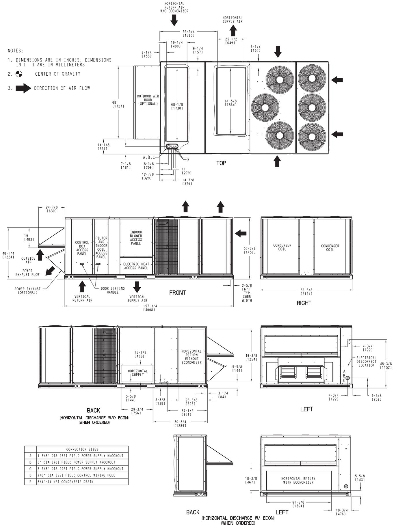
Fig. 4 — Unit Dimensional Drawing — RAH300 and 303
