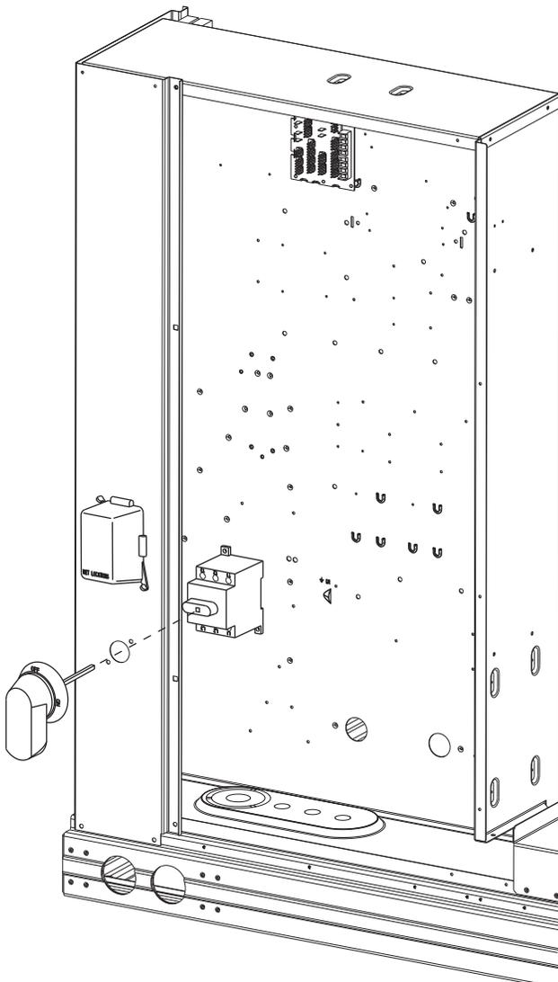
Fig. 21 — Handle and Shaft Assembly for NFD
