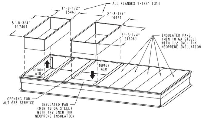
Fig. 10 — Roof Curb Details — RAH300 and 303
