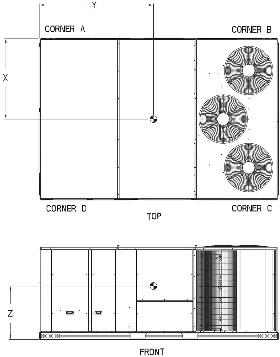
Fig. 2 — Unit Dimensional Drawing — RAH181 and 183 (cont)
