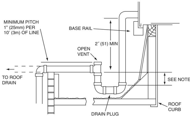
NOTE: Trap should be deep enough to offset maximum unit static difference. A 4" (102) trap is recommended
