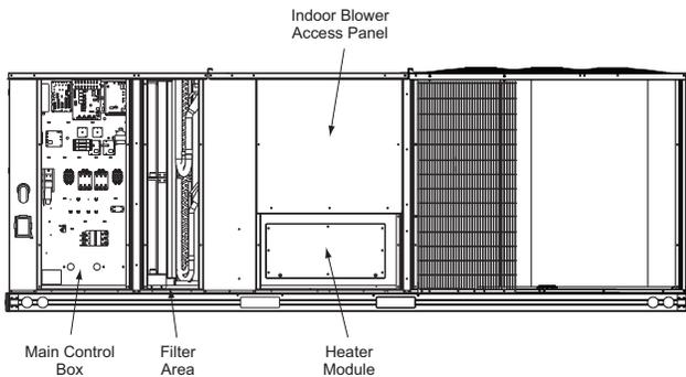
**Fig. 30 — Typical Component Location**
