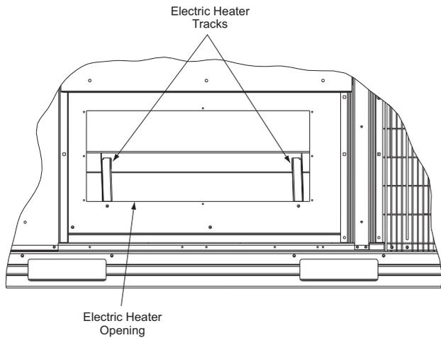
**Fig. 31 — Electric Heater Compartment (Cover Removed)**
