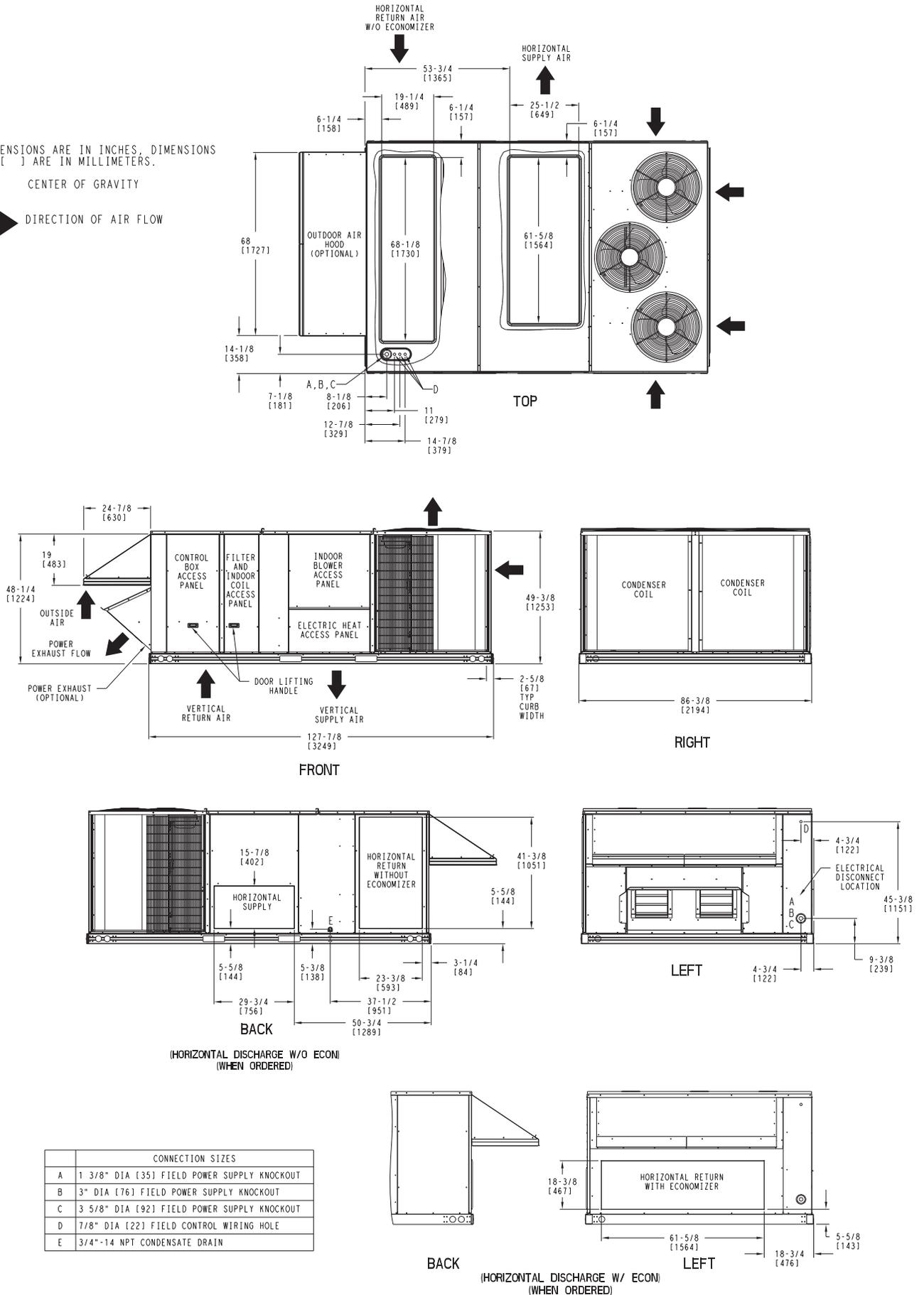
Fig. 2 — Unit Dimensional Drawing — RAH181 and 183
