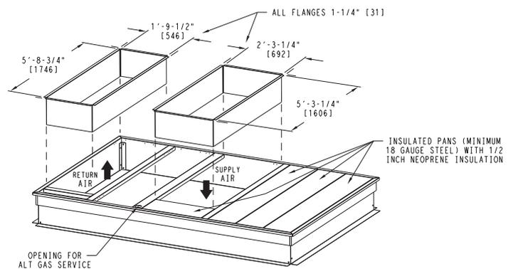
Fig 8 — Roof Curb Details — RAH181 and 183
