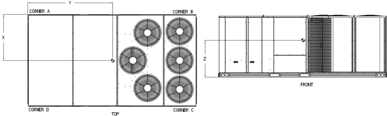
Fig. 4 — Unit Dimensional Drawing — RAH300 and 303 (cont)
