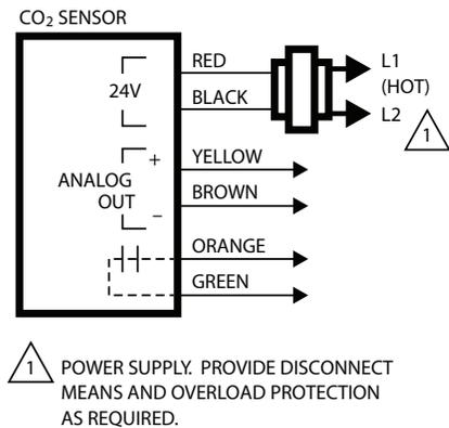
**Fig. 37 — CO<sub>2</sub> Sensor Wiring**
