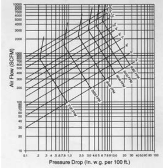
**STRAIGHT RUN** \* FD 72-R1 Test Code of the Air Diffusion Council. Friction loss is computed in inches of water gauge per 100 ft. of straight duct. By using CFM or FPM values for a given duct dimension, the friction loss can be determined. Conversion of CFM to FPM also can be made.
