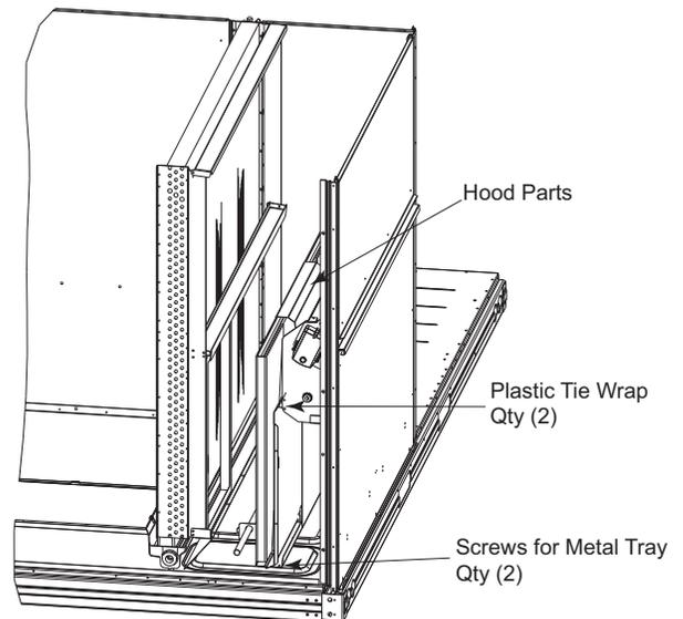
**Fig. 20 — Two-Position Damper Hood Package Location**
