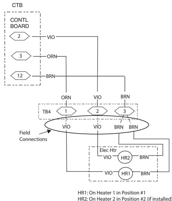
**Fig. 58 — Accessory Electric Heater Control Connections**
