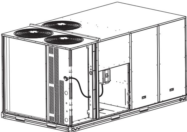
**Fig. 37 — Conduit into Factory Option Disconnect**
