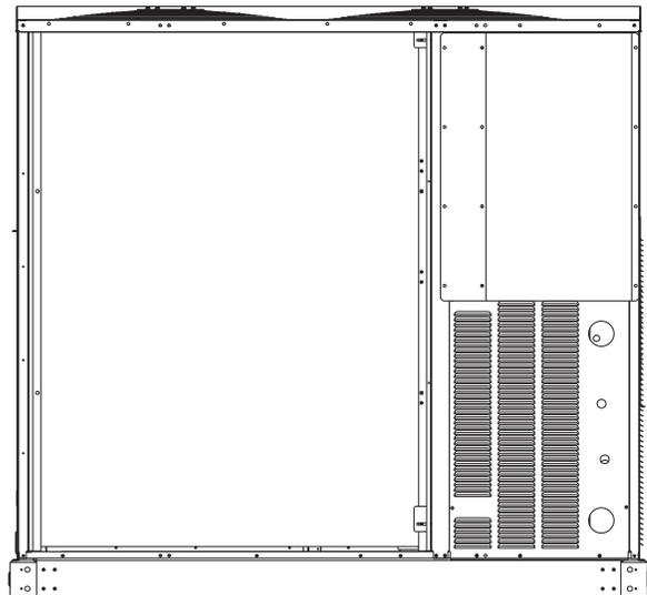
**Fig. 40 — Mounting Position for Field Disconnects (over 100A)**
