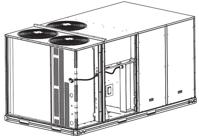
**Fig. 39 — Conduit into Single Point Box**
