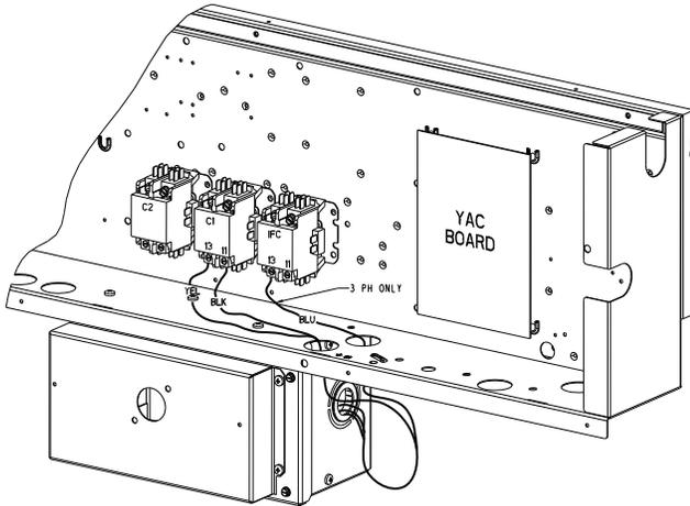
**Fig. 28 — Location of Non-Fused Disconnect Enclosure**
