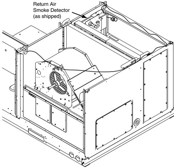
**Fig. 70 — Return Air Smoke Detector; Shipping Position**
