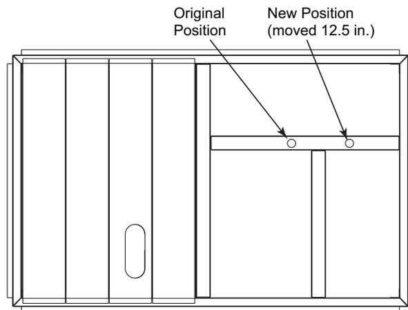
**Fig. 11 — Alternative Condensate Drain Hole Positions**
