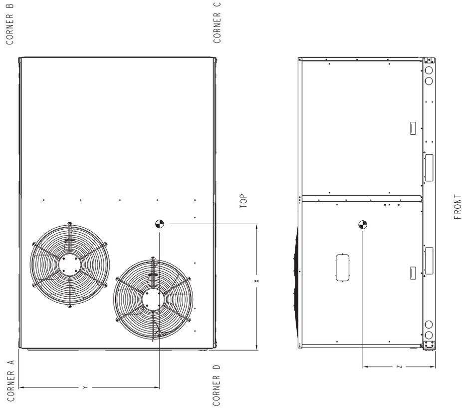
Fig. 2 — Unit Dimensional Drawing — RAS089-120 (cont)
