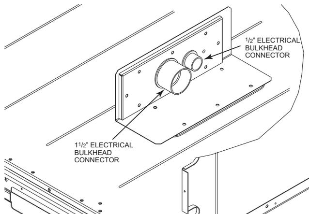
**Fig. 50 — Thru-the Base Option, Shipping Position**
