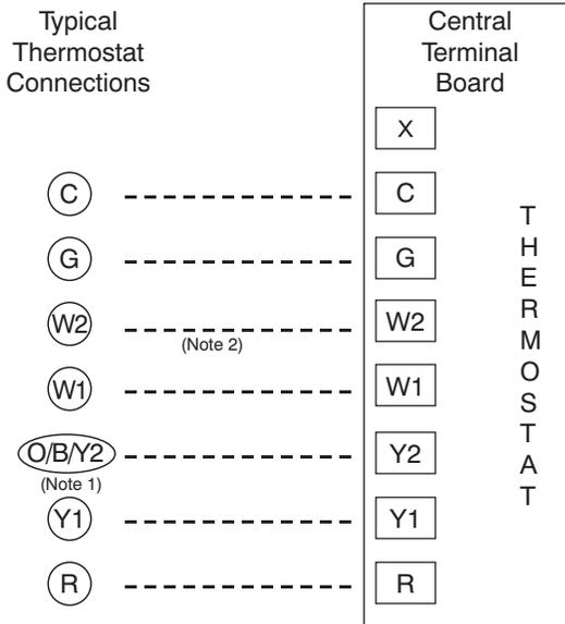
Note 1: Typical multi-function marking. Follow manufacturer's configuration instructions to select Y2. Do not configure for O output.
