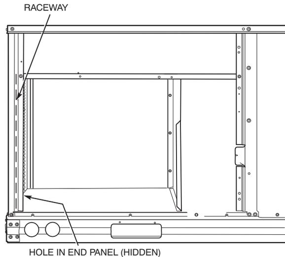
**Fig. 36 — Field Control Wiring Raceway**
