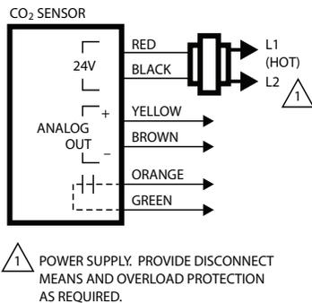
**Fig. 67 — CO<sub>2</sub> Sensor Wiring**
