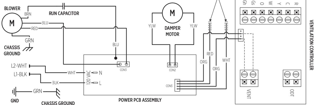
**FIGURE 16 – MODEL 8140NC INTERNAL SCHEMATIC**
