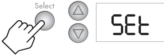
Throughout the Set Up Menu, the ▲ and ▼ buttons are used to change values, the **Select** button is used enter the value and move on to the next Set Up Menu item.
