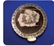
• After 300 cycles: Thermal grease voids and pumps out
