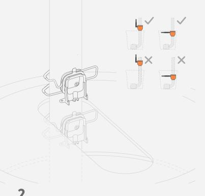
The bottom of Sumpie needs to be able to see the water level in your sump pit. Snap the mounting holster onto to the pipe leading out of your sump pit. If the lid has a hole that Sumpie can see through, attach the mounting holster directly above the hole. If there isn't a hole, attach Sumpie directly below the lid inside the pit.
